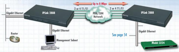
**The Model 2888** provides point-to-point high-bandwidth Ethernet/IP connectivity over TDM-based T1/E1 circuits.
